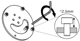
**2b** Insert U-Frame on screws
